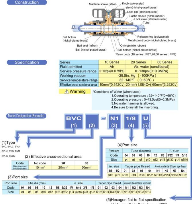
U: Hexagon flat-to-flat inch spec. (NPT) No code: Hexagon flat-to-flat mm spec.
